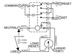
**Contact Ratings:** SPDT dry relay contacts, 10 A, 125 VAC.
